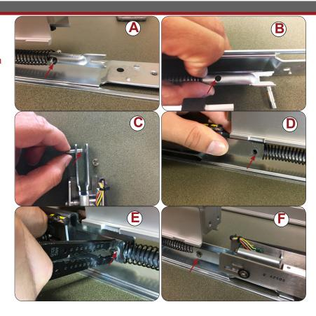
**9.** Once the kit is secure with the pin, lift up and insert back screw into the bottom dogging hole. Do not tighten until device is assembled.
