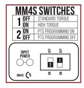
Input Voltage: 24VDC +/- 10%Wire gauge: Minimum 18 gauge
