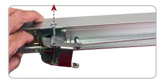
\*First Choice Devices Only: Cut down Back Activating Bracket to remove Dogging Extension.
