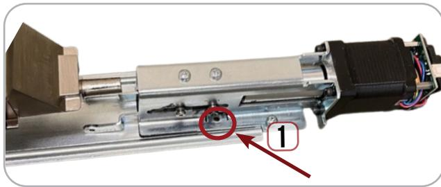
4. Turn full assembly to the side & install (E) **Screws** from underneath to secure motor kit to Base Rail.
