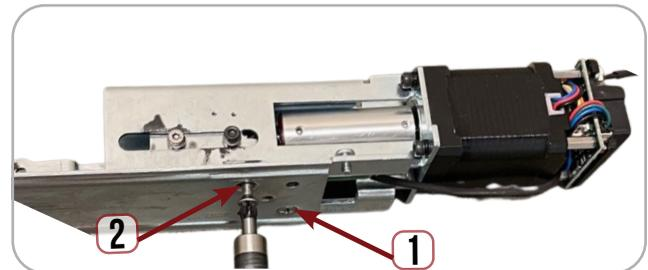
5. Slide the (B) **Connecting Bracket** over the Dogging post at the end of the push pad. Next, move **Attaching Arms** on motor kit up to line up with holes on **B Bracket**.
