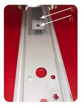
FOR HOLE #2, YOU'LL NEED TO START LOOSING IT BY USING VISE GRIPS OR A NEEDLE NOSE PLIERS & WORK THE SCREW LOOSE.
