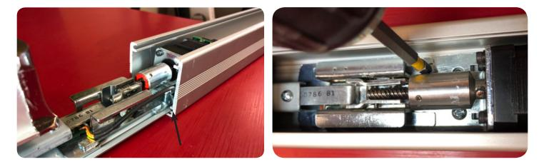
9. NEXT, HOOK UP TO POWER AND SET THE PUSH-TO-SET ADJUSTMENT. FOLLOW STEPS BELOW TO SET, REMEMBERING TO TURN THE PROGRAMMING SWITCH TO THE OFF POSITION WHEN COMPLETED.
