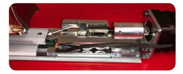
5. INSTALL BOTH (40786) SCREWS & (40351) LOCK WASHERS PARTIALLY, SO THE BASERAIL CAN STILL SLIDE BACK INTO THE HOUSING.
