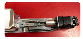
6 INSTALL (40064) SCREW TO SECURE ATTACHING BRACKET TO CONNECTING ROD
