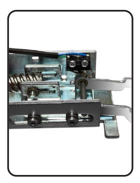
2. Guide **REX Cable** along **Motor Mount** and secure through cutouts using **Zip Ties** provided.
