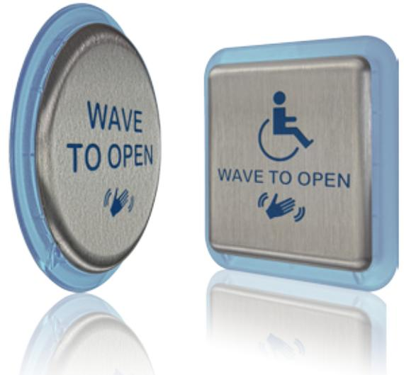
The MS21 is a state-of-the-art touchless activation plate that utilizes capacitance technology to detect and trigger activation in automatic doors. The low profile, hands-free MS21 includes a stainless steel faceplate and illuminated LED mounting ring for maximum durability and visibility. Other innovative features include adjustable detection zones, audible alerts, NEMA 4-rated enclosure and customizable faceplate text and logos.
