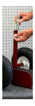
1 With the axel installed through the axel tube, the wheels installed and secured with cotter pins, slide the short 3/4" bar into the upright tube and install with a detent pin as shown.
