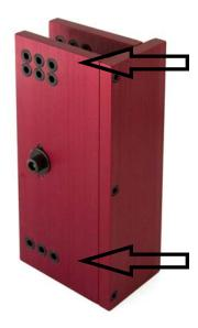
Drill three 1/4" holes through the door. Enlarge the center hole to 3/4" with the use of a hole saw. Use top set of holes.
