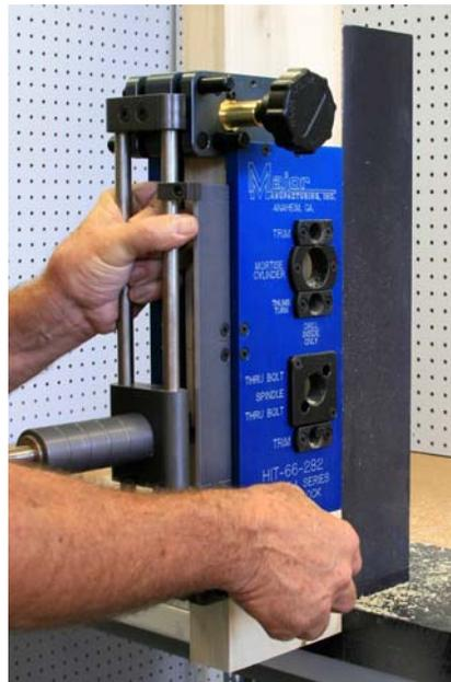
When all holes have been drilled, remove the template from the door.
