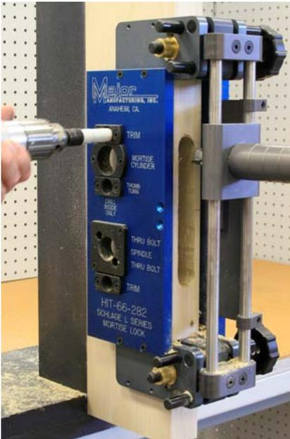
Thru bolt holes for the trim being drilled half way from both sides of the door.
