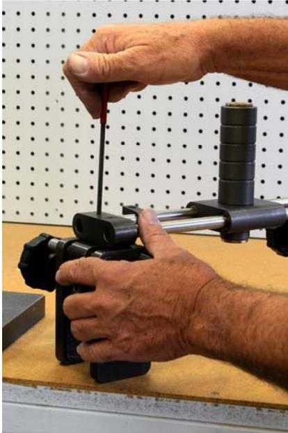
Attach the mortiser attachment to the HIT-66 clamp set using the supplied 1/4-20 x 1-1/2" socket screws. The mortiser is held to the HIT-66 clamp system with two screws on top and two on the bottom. Leave all screws loose at this time.
