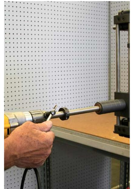
Attach a drill motor to the cutter shaft and tighten the chuck.
