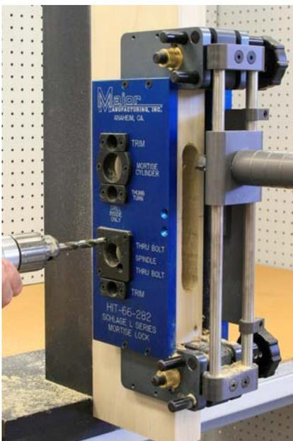
Thru bolt holes being drilled on both sides of the door.
