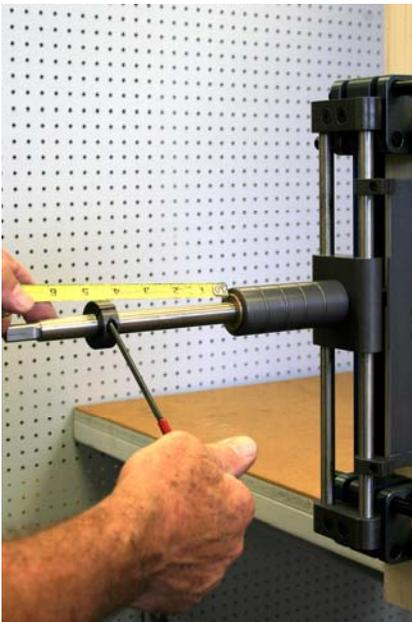
Touch the bit to the door edge and measure the depth that you want to drill. Tighten the stop collar, this will limit the depth of the mortise pocket.
