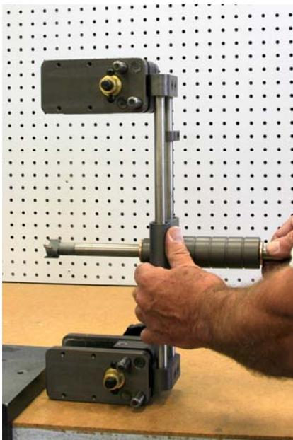
Slide the mortise bit into the unit and slide the stop collar on the end of the shaft.
