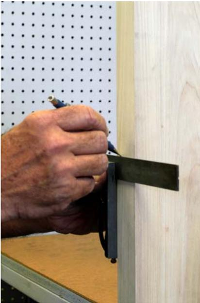
Using a pencil, establish the centerline of the mortise pocket as shown at left. Put the mortise unit on the door and align as shown on the right. Tighten the clamp knobs top and bottom alternating between the top and bottom clamp. Do not attempt to tighten one clamp all the way at once.
