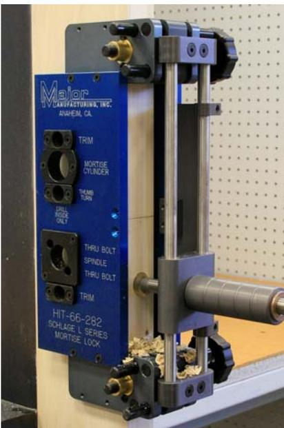
Start at the bottom and drill a hole to depth. Back out the bit to clear the chips, do not attempt to drill the hole to depth all at once. Use a moderate drill speed 350 to 500 rpm.
