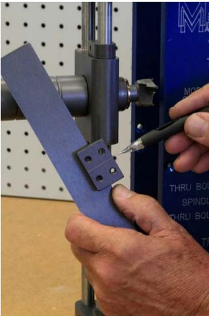
The next part to attach to the template is the alignment guide. When installed, it will align the mortise pocket to the drill guide. Notice the scribe mark in the picture at the left. The guide can be attached to either template, it is attached with two 10-32 x 3/4" flat head socket screws.
