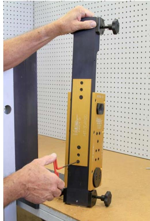
If retrofitting, install the HIT-30AR20 to the clamp and align it in the existing faceplate cutout.
