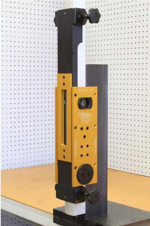
For a new install, locate the template at the desired height and drill a starting hole for the router.
