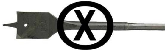
Shown above is a spade or paddle type bit. Do not attempt to use this in any drill guide. There is no bearing surface and you will jam the bit.
