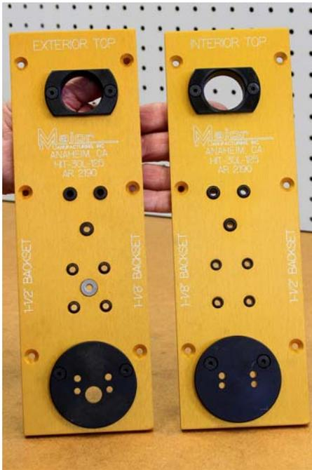
There are two templates in the HIT-30L-125 template set. One is an outside template and the other for the inside. Both templates will prep either a 1-1/8" or 1-1/2" template. Reversible for RH or LH doors.
