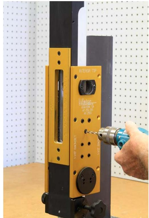
There are three holes inside and outside to drill next. The factory template calls for a .196 diameter drill bit. Our drill guides will accept a 13/64" twist drill, a lot easier to find in the field. The bottom holes shown being drilled on the right is a pilot hole that will be drilled later.
