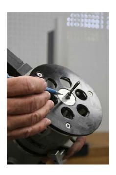
Your router needs to be equipped with a 3/8" outside diameter template guide mounted in its base. Failure to use a template guide will cause the opening being routed to be too large and will damage your HIT-41 template.
