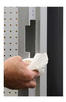
Clean the area of left over cutting lube and chips. Be sure to use a brush to remove the chips, they are sharp!
