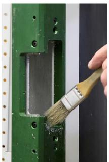
After making the first pass, brush away the chips and make a second clean up pass. Use the same procedure as before.
