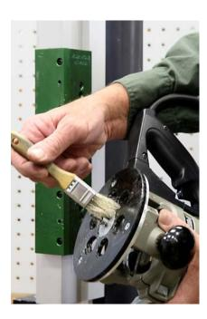
Brush the aluminum chips from the router guide to prepare for the second clean up pass.
