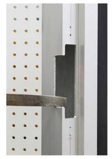
Don't forget to square off the corners for the lip area in front of the front of the frame, the router will leave these round.
