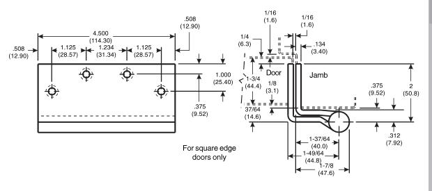
NOTE: This hinge alters the normal pivot point of door. For door closers, friction or overhead door holders, to be used in conjunction with this hinge, consult manufacturer of the device to be used for application details.
