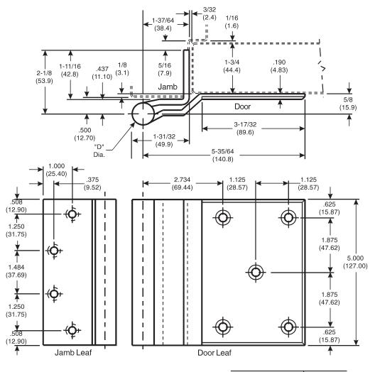
NOTE: This hinge alters the normal pivot point of door. For door closers, friction or overhead door holders, to be used in conjunction with this hinge, consult manufacturer of the device to be used for application details.
