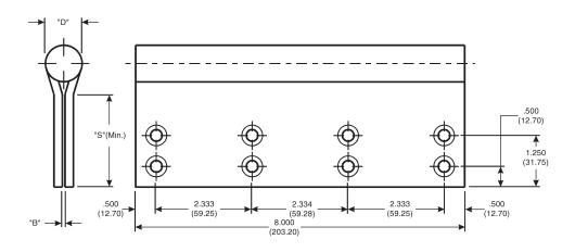
The above pattern is for 1-3/4" to 2-1/4" thick doors; For doors greater than 2-1/4" thick see template 046B
