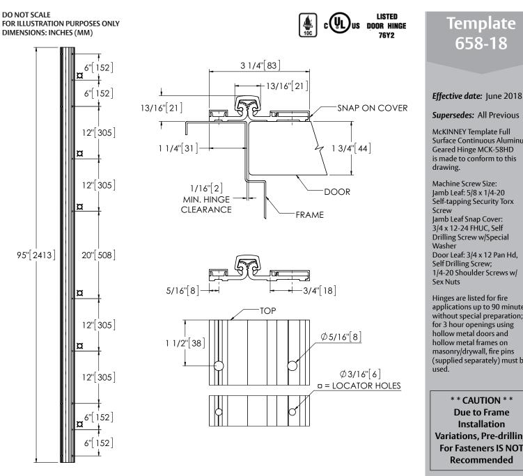
Surface Continuous Aluminum Geared Hinge MCK-58HD is made to conform to this
