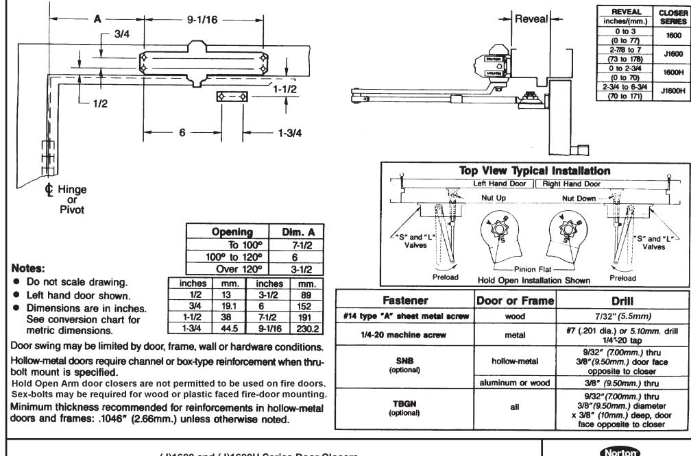
(J)1600 and (J)1600H Series Door Closers Top Jamb Application Non Hold Open or Hold Open Arm Individually Sized Units 3 and 4 & Multi-size Units 1-6
