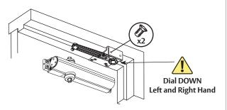
6. Place main arm on closer spindle and rotate.
