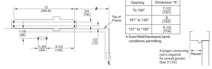
2. Mount closer to frame. 3a. Remove dial from 3b. Install separate arms. Hold Open arm. MM B an B x2 Flat Dial DOWN Left and Right Hand RH and LH: Position flat at S 4. Connect arms, preload spring 5. Set Hold Open. Keep door open in position until dial screw secures dial. and tighten set screw.  $(\mathbf{i})$ 1st 1st Rotating arm 70° - 180' 90 preloads closer spring power. 3rd 1st 2nd A 3rd 2nd 3rd 2nd Rotate elbow until LH: Counter RH: Hold Open arm is clockwise to Clockwise
