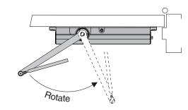
7. Remove arm and attach as shown.
