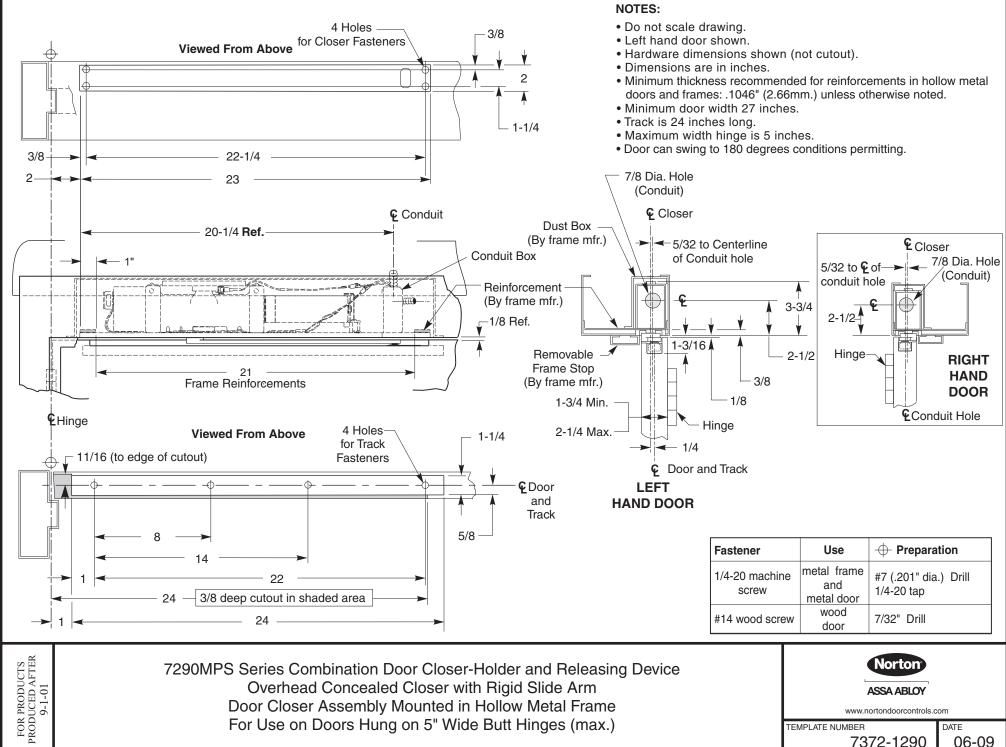
7290MPS Series Combination Door Closer-Holder and Releasing Device Overhead Concealed Closer with Rigid Slide Arm Door Closer Assembly Mounted in Hollow Metal Frame For Use on Doors Hung on 5" Wide Butt Hinges (max.)
