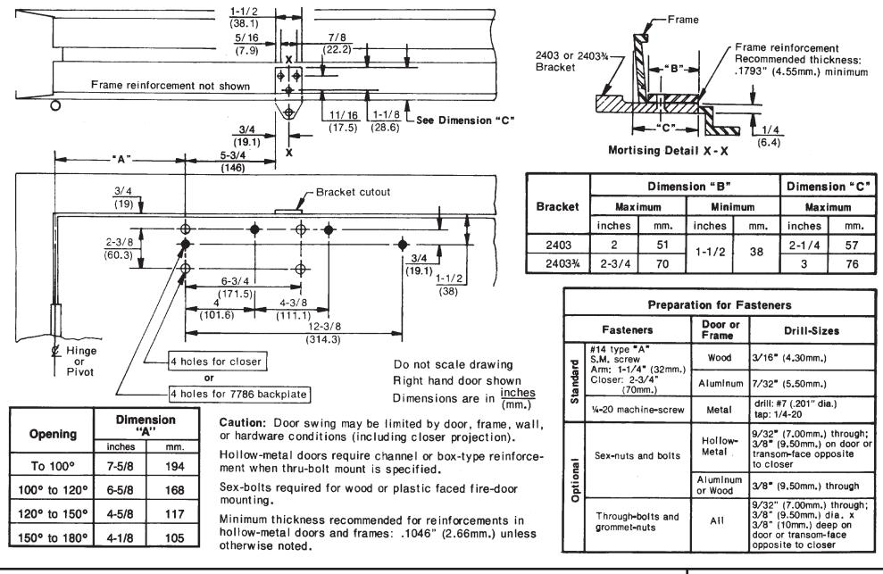
7500, 7700, 7700COU and 7700TEL Series Door Closers With 2403 or 2403-3/4 Bracket With or Without 7786 Backplate Regular Arm Installation With Non Hold Open Arm
