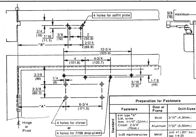
Do not scale drawing Left hand door shown Dimensions are in  $\frac{\text{inches}}{(\text{mm.})}$
