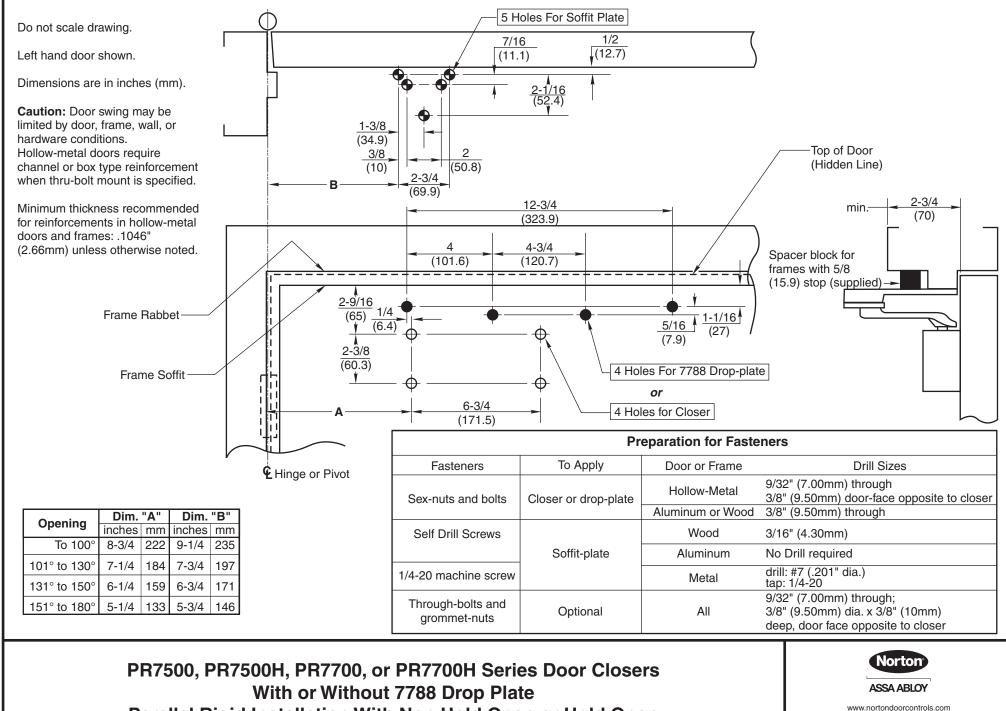
Parallel Rigid Installation With Non Hold Open or Hold Open
