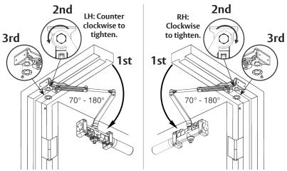
You've now installed the **7500H Hold Open Closer - Parallel Arm.**
