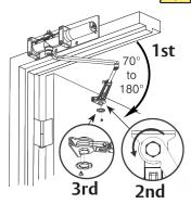
LH: Counter clockwise to tighten.
