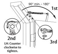
You've installed the **7500H Hold Open Closer - Regular Arm.**
