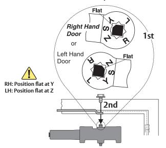
6. Connect arms, preload and tighten set screw.
