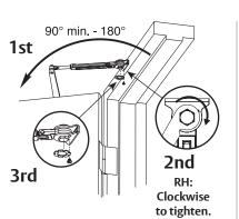
Keep door open in position until dial screw secures dial.
