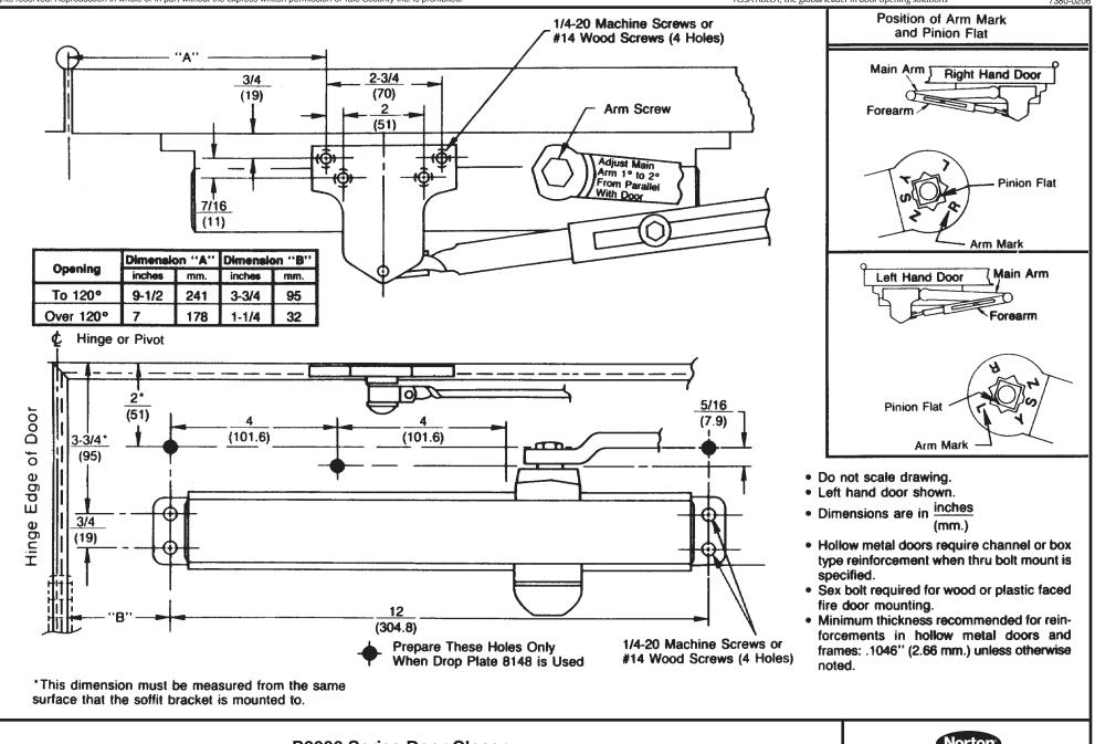
P8000 Series Door Closer Parallel Arm With 2018D For Narrow or Blade Stop Application With or Without 8148 Drop Plate P8100, P8300, and P8500 Sizes 1 Thru 6
