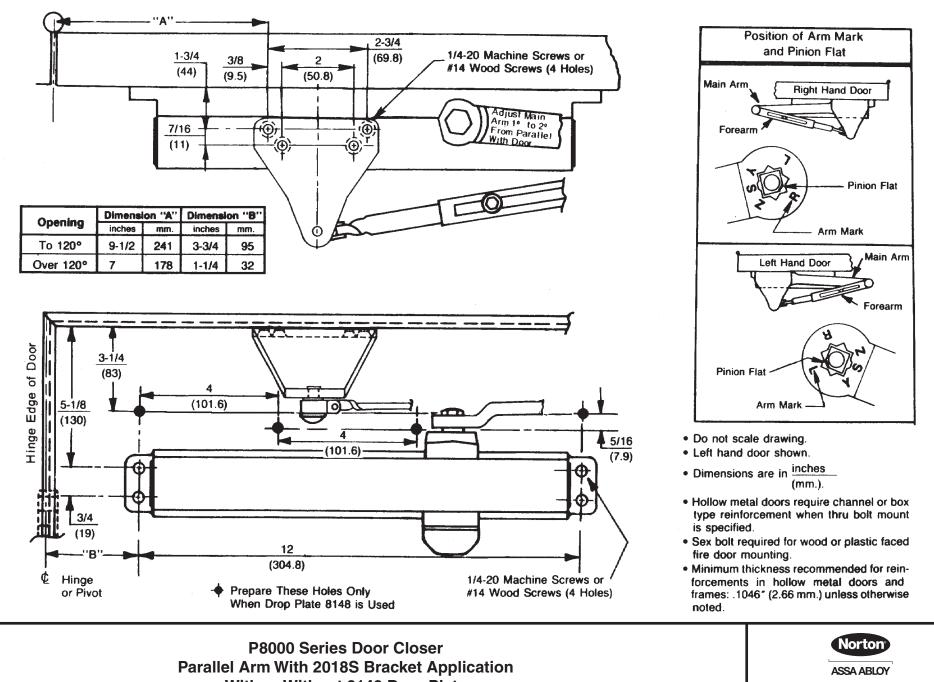
With or Without 8148 Drop Plate P8100, P8300, and P8500 Sizes 1 Thru 6
