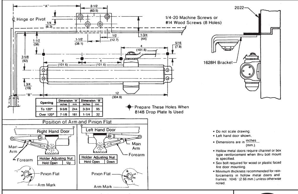
P8000H Series Door Closers Parallel Hold Open With 2022 x 1628H Bracket P8100H, P8300H, and P8500H Sizes 1 thru 6
