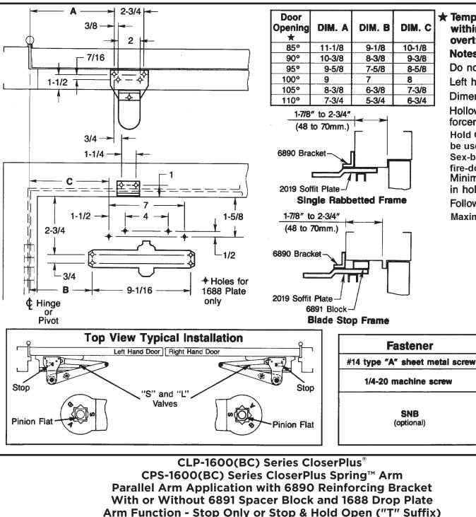
Power Sizes 1-6, 3BC, or 4BC Approved 2022-02-25 ★ Template dimensions are for hold-open/door stop within ±2° of charted door openings. Doors may overtravel up to 5° beyond the rest position. Notes:
