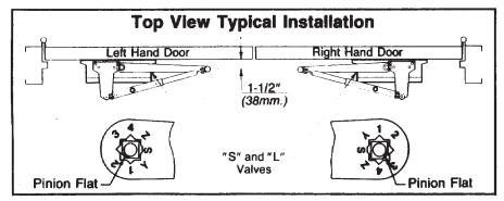
(P)1680 Series Door Closers With Low Profile Arm Parallel Arm Application With or Without 1688 Drop Plate Non Hold Open Arm Individually Sized Units 3 and 4 & Multi-size Unit 1-6
