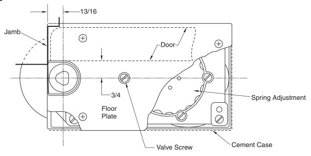
Closing speed can be adjusted to suit local conditions and requirements. With a screw driver turn the adjustment screw that projects through the floor plate or threshold, either in or out as the case may be until the desired action is attained. Turn this valve
