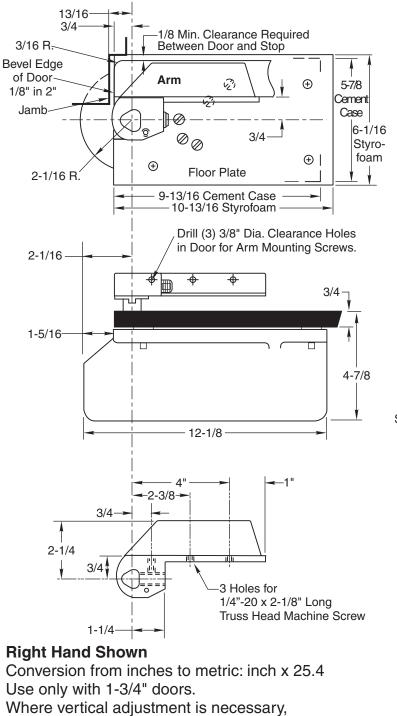
two (2) 1/16" thick shims are provided to be placed between arm and torque washer.
