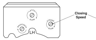
Closing speeds can be adjusted to suit local conditions and requirements. Label on closer face designates the purpose of each adjustment screw.
