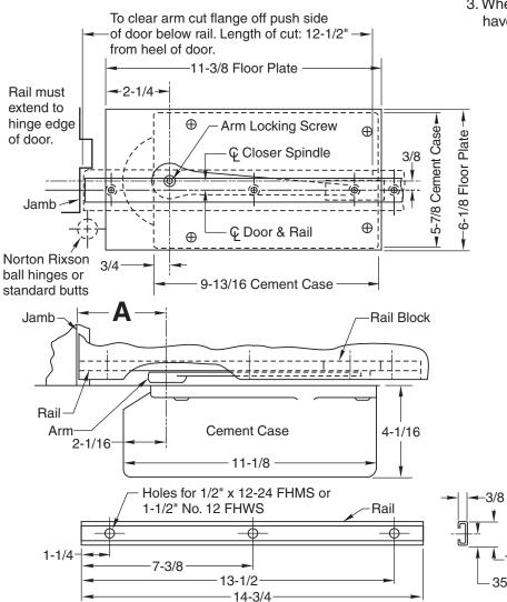
DIMENSION "A" SHOWN IN THE TABLES ARE FOR 1-3/4" THICK DOORS ONLY-CONTACT THE FACTORY FOR DOORS OTHER THAN 1-3/4"
