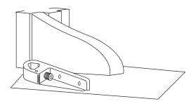
CAUTION: Closer is shipped with "closing speed" valve down. DO NOT FORCE VALVE DOWN.
