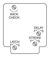
Closing speeds can be adjusted to suit local conditions and requirements. Label on closer face designates the purpose of each adjustment screw. Adjustments are for speed control.
