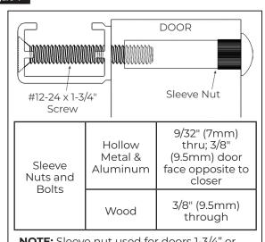
**NOTE:** Sleeve nut used for doors 1-3/4" or greater. For doors less than 1-3/4", sleeve nut body will need to be shortened.
