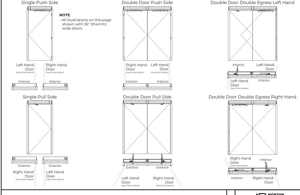
**6051 Series Template** for 36"-48" wide door shown with up to 5" Butt Hinges Reveal of 1/8" to 3" Maximum Opening of 110°
