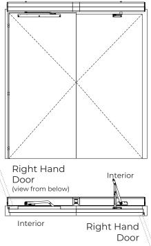
D6001DER2 Series Template shown on pairs of 36", 38", 40", 42", 44", 46" and 48" frames shown with up to 5" Butt Hinges Reveal of 4-3/4" (121) to 7-3/8" (187) on Push and Pull sides Maximum Opening of 100° NORTON RIXSON
