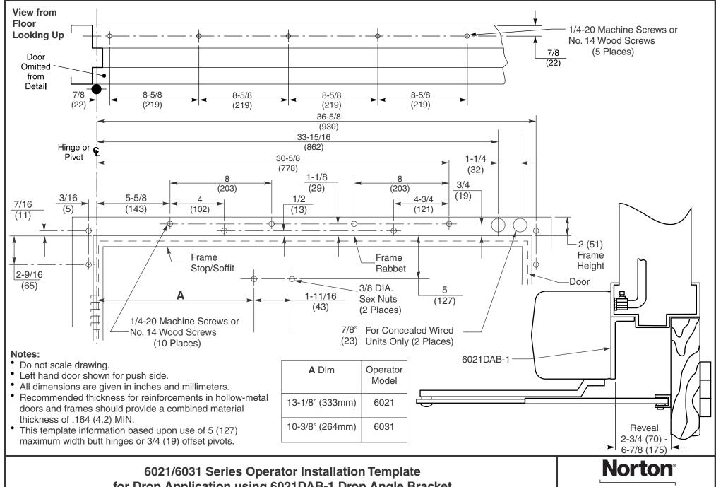
6021/6031 Series Operator Installation Template for Drop Application using 6021DAB-1 Drop Angle Bracket on 36" wide doors For Reveal of 2-3/4" (70mm) to 6-7/8" (175mm) ASSA ABLOY www.nortondoorcontrols.com
