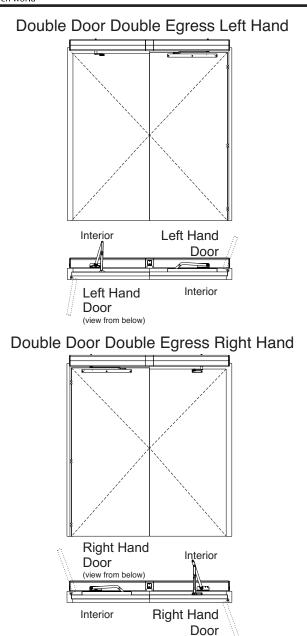
6021 Series Template shown on 36" and 42" frames shown with up to 5" Butt Hinges Maximum reveal of 6-7/8" and Maximum of 110 degrees of opening
