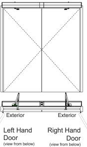
6051 Series Template for 36" wide door minimum shown with up to 5" Butt Hinges Reveal of 1/8" to 3" Maximum Opening of 110 degrees
