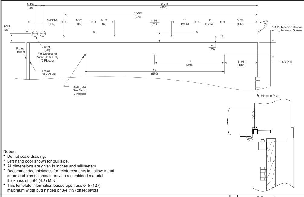
6051 Series Template for 36" wide door minimum shown with up to 5" Butt Hinges Reveal of 1/8" to 3" Maximum Opening of 110 degrees Norton
