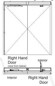
6061 Series Template shown on 36" and 42" frames shown with up to 5" Butt Hinges Reveal of 2-1/4" to 4-3/4" and Opening of 85 to 110 degrees Norton®
