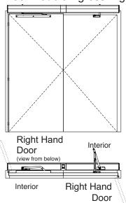
6071 Series Template shown on 36" and 42" frames shown with up to 5" Butt Hinges Reveal of 4-13/16" to 7-3/8" and Opening of 85 to 110 degrees
