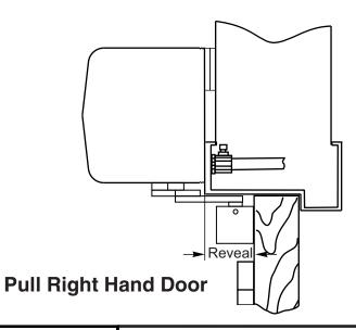
**D6001DE-R Series Operator Installation Template** for Double Door Double Egress Frame with Right Hand Doors on 36"(914mm), 42"(1067mm), or 48"(1219mm) leafs (shown on 36" wide leafs) For Reveal of 1/8" (3mm) to 3" (76mm) for Pull Side Door and 2-1/4" (57mm) to 4-3/4" (121mm) for Push Side Door
