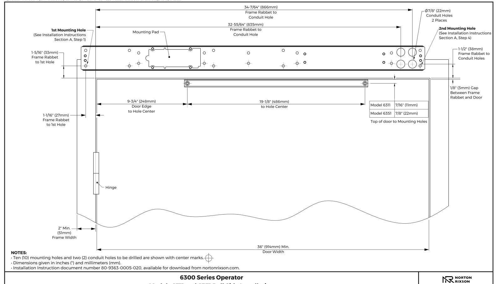
Models 6311 and 6351 Pull Side Installation 36-48" Door Width, 90-250 lb. Door Weight 180° Max Open Angle Approved 2024-04-01
