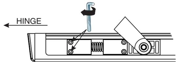
Open door to maximum desired swing minus 5° and hold. Slide spring cushion stop assembly against slider assembly and secure to track using 5/64" or 2mm wrench.
