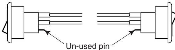
SHO switch in closed position. Closer in hold open.
