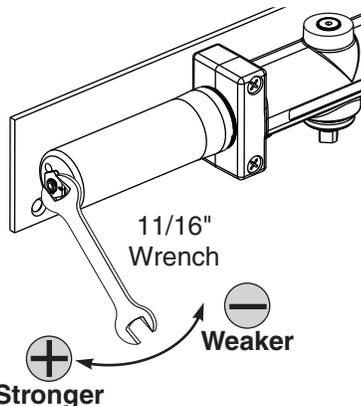
Slowly increase closer power until door closes consistently. A closer set to the ADA required 5 lbs opening force may not be strong enough to close the door due to latching hardware, air pressure, or frame issues.
