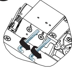
Fully close Latch & Sweep Valves with 1/8" wrench provided.
