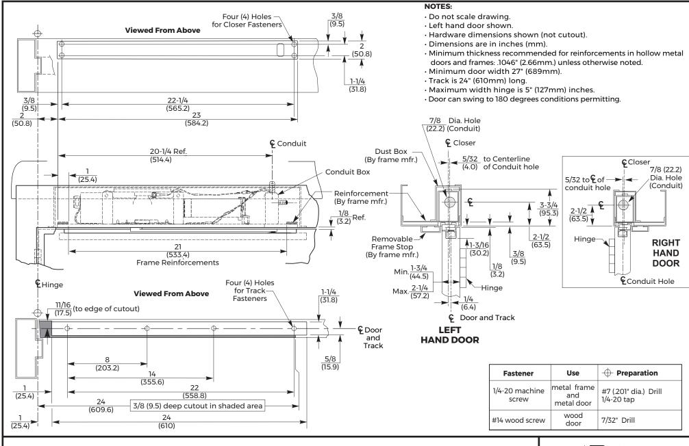
7290MPS Series Combination Door Closer-Holder and Releasing Device Overhead Concealed Closer with Rigid Slide Arm Door Closer Assembly Mounted in Hollow Metal Frame For Use on Doors Hung on 5" Wide Butt Hinges (max.) ASSA ABLOY
