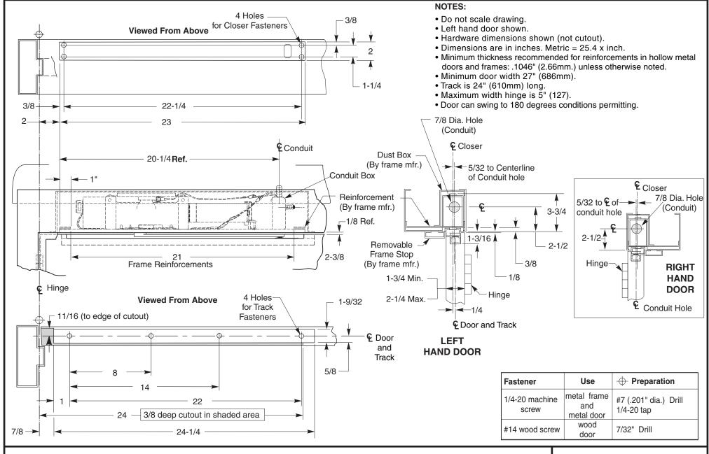
7290MPS x 790 Fire Bloc Series Combination Door Closer Holder and Releasing Device Overhead Concealed Closer with Rigid Slide Arm Door Closer Assembly Mounted in Hollow Metal Frame For Use on Doors Hung on 5" Wide Butt Hinges (max.) NORTON
