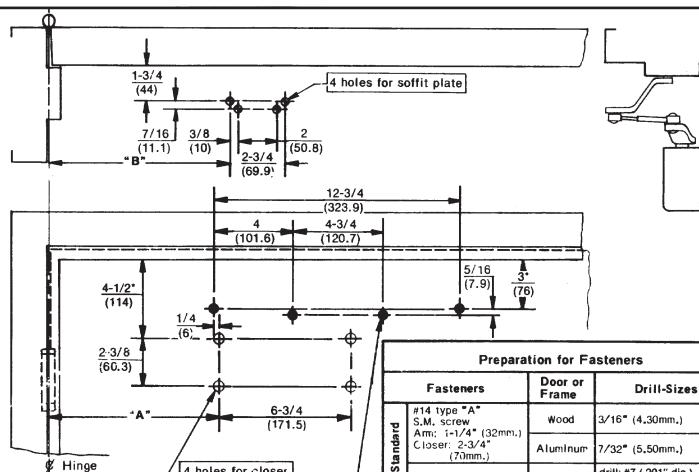
Do not scale drawing Left hand door shown Dimensions are in  $\frac{\text{inches}}{(mm.)}$
