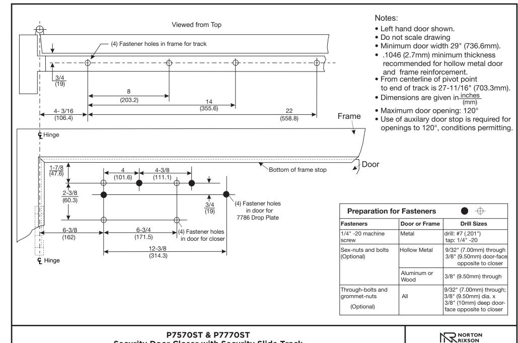
**P7570ST & P7770ST Security Door Closer with Security Slide Track** With or Without 7786 Drop Plate For Use on Doors with 4" or 5" Wide Butt Hinges Non-Hold Open, Stop Mounted Installation
