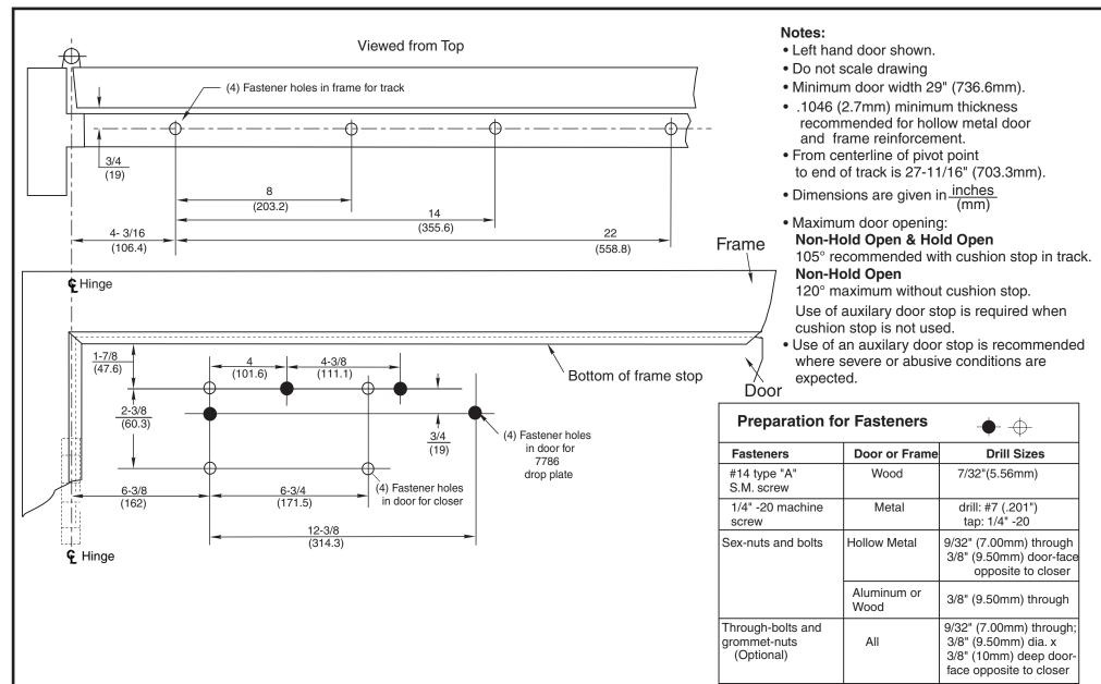
PS7540ST and PS7740ST Non Hold Open-Stop Mounted Installation PS7540STH and PS7740STH Hold Open-Stop Mounted Installation **Door Closer with Slide Track** With or Without 7786 Drop Plate For Use on Doors with 4½" or 5" Wide Butt Hinges
