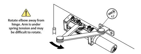
You've installed the 7570/7770 Security Non Hold Open Closer - Regular Arm.
