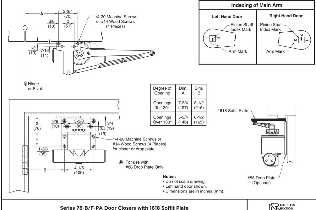
**Non-Hold Open Parallel Arm Installation** With or Without No. 88 Drop Plate Closer Sizes 78-B/D-PA or 78-E/F-PA
