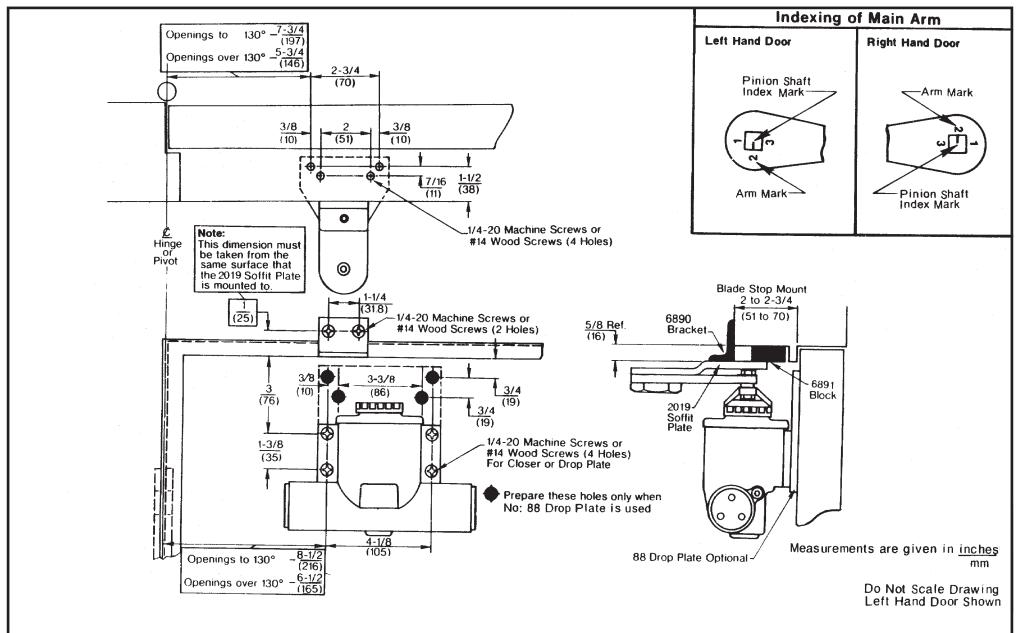
Series 78-B/F-(PRA or PHA) Door Closers With 6890 Support Bracket & 6891 Spacer Block Non Hold-Open or Hold-Open Parallel Rigid Arm Installation With or Without No. 88 Drop Plate Closer Sizes 78-B/D or 78-E/F NORTON
